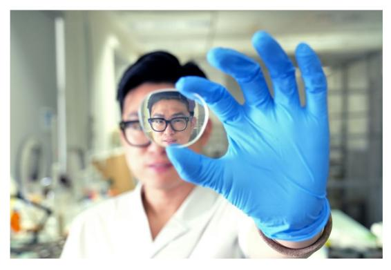
The new type of coating – when applied on a plastic surface, prevents fogging and 'self-cleans', overcoming the need for frequent reapplications (Image: NTU Singapore)
